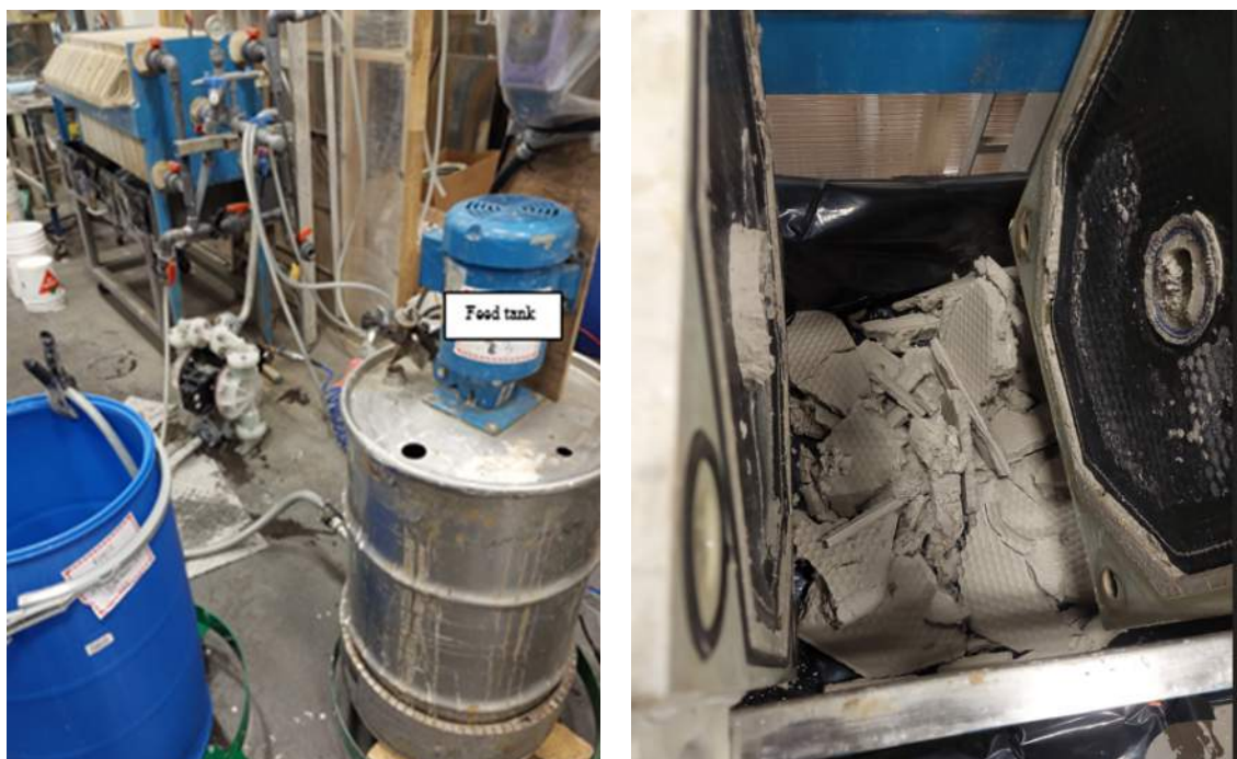
Figure 13-5: Filtration Equipment and Leach Residue Cake
