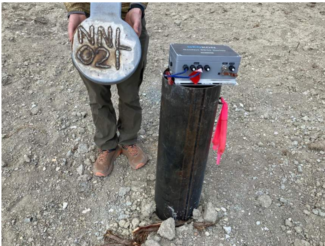
Figure 12-2: Reverse Circulation Drill Hole NNL-021 Completed as a Piezometer Well
